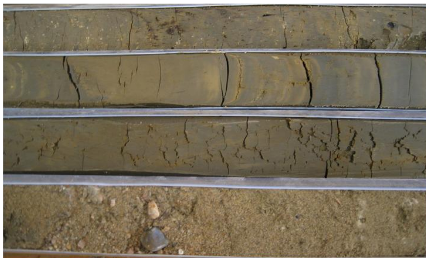
Fig. 2.15 Sections of soil cores , ranging from fill, sandy clay, clay, through sand with pieces of gravel. Sampling by means of CPTU device equipped with separate sampler.
